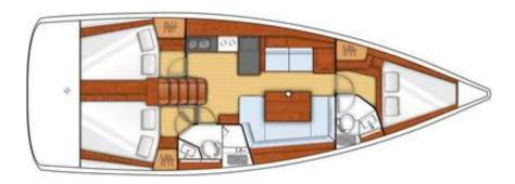
Length overall: 12,38 m Beam: 4,20 m Draft: 2,05 m 40 HP Engine: Fuel capacity: 200 lt Water capacity: 570 lt 41,7 m<sup>2</sup> Sail area: 8 Accommodation:
